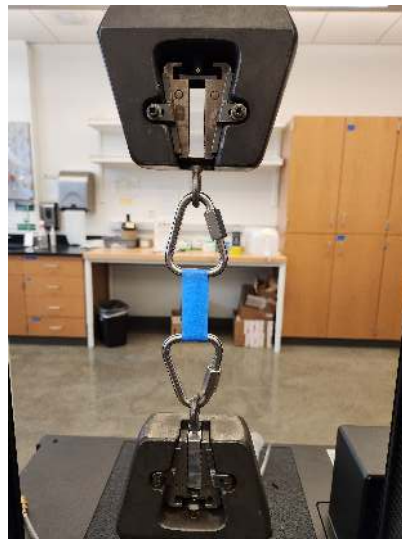
Figure 81: Break Banding Apparatus
