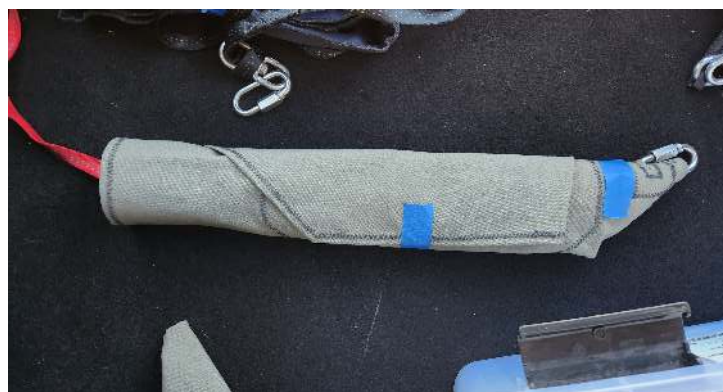
Figure 31: Shock Cord Wrapping Method
