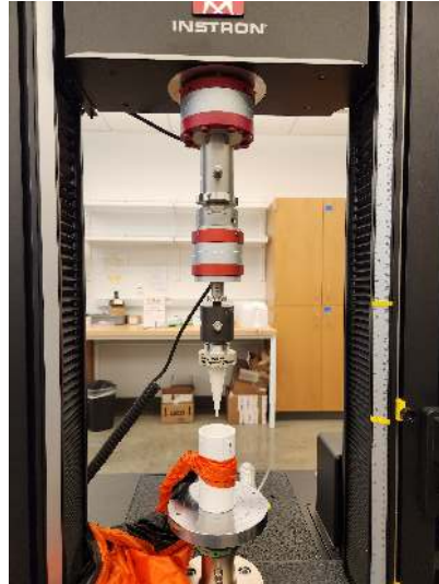
Figure 79: Parachute Durability Apparatus
