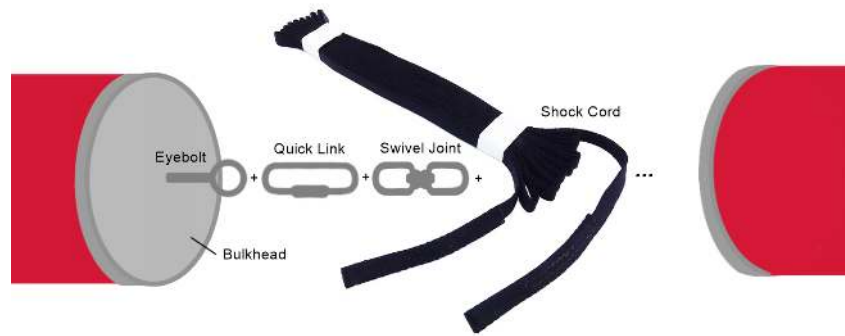
Figure 28: Hardware Diagram of Linkage Order
