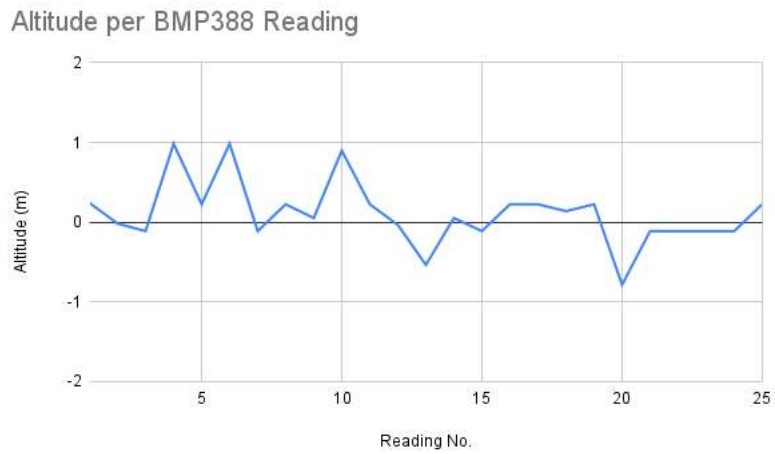
Figure 122: Altitude Readings in meters from BMP388
