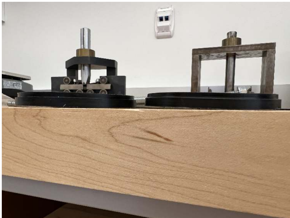
Figure 113: Permanent Deformation of Delrin Bulkheads After Released from 15 kN Test
