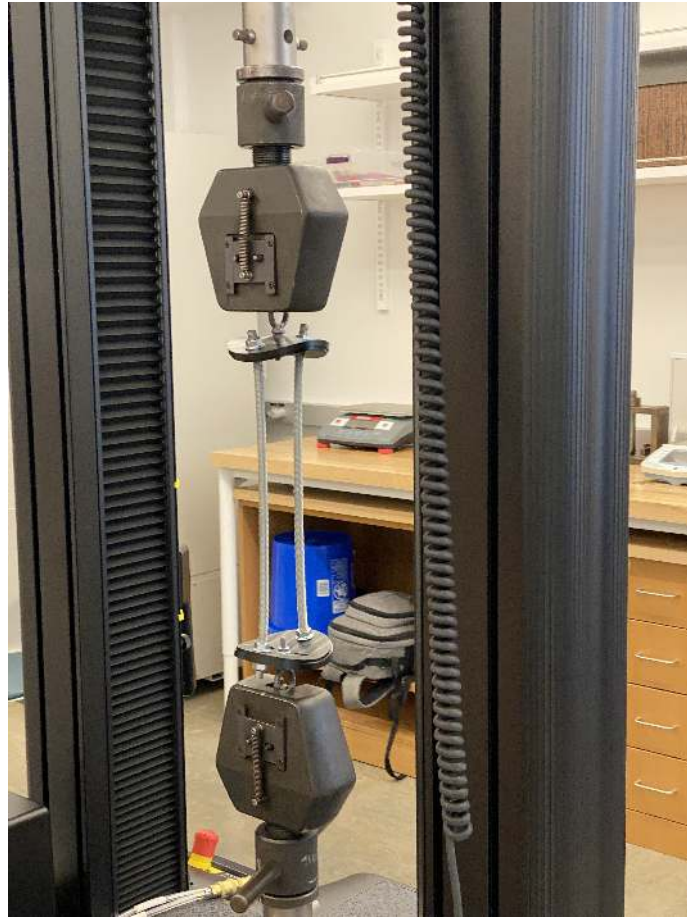
Figure 112: Visible Bending Of Bulkhead Testing Sample With 15 kN Applied
